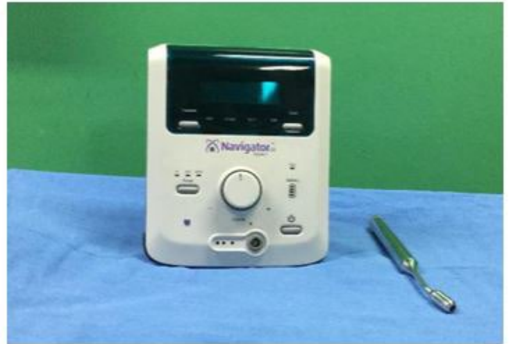
Figure 7: Showing Wireless gamma detection probe and portable display console for SLNB using a radioactive tracer.
