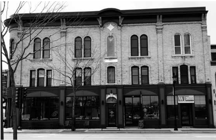
3.5. Flanagan Building in downtown Oconomowoc, WI, which was constructed with Fulmer brick. The building is unusual because of its arched brick window casings. The Fulmer brickyard was the only local brickyard where beveled brick molds were used to make the bricks necessary to construct arched window casings.
